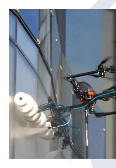
**Increased Efficiency:** Drones can autonomously perform high-altitude cleaning tasks. With precise navigation and smart planning systems, they can quickly cover large areas, avoiding the extensive time and labor required for scaffolding or basket setups, thus greatly improving work efficiency.
